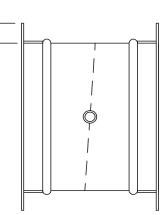
Equal Leg Angles are available. They are welded to frames at intermittent spacing and caulked between welds. Flange Height "D" varies with Damper Diameter.
